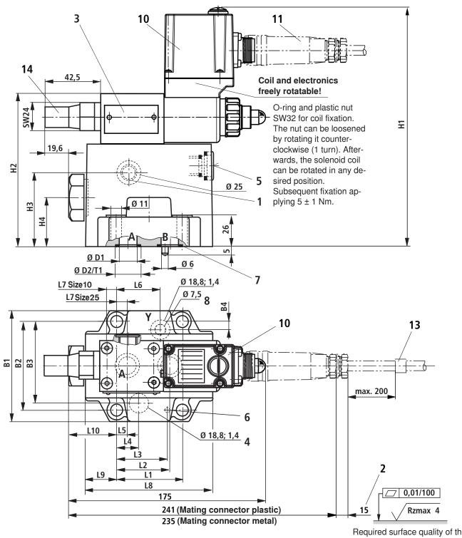
Required surface quality of the valve mounting face
