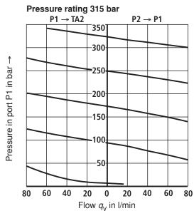
Min. set pressure in dependence upon the flow at zero command value
