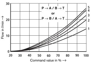
30 I/min nominal flow at 10 bar valve pressure differential
