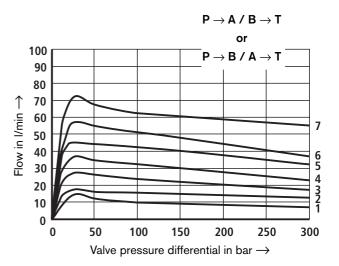
If the performance limits are exceeded then flow forces occur which lead to uncontrolled spool movements.
