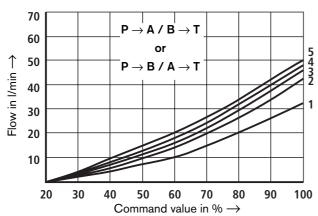
60 I/min nominal flow at 10 bar valve pressure differential
