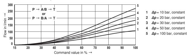
125 I/min rated flow at 10 bar valve pressure differential
