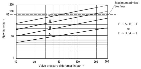
Observe the maximum admissible flow of 80 l/min!
