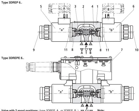
Valve with 2 spool positions: (type 3DREP..A.. or 3DREP..B..) The function of this valve design corresponds basically to the valve with 3 spool positions. The 2 spool position valves are, however, only equipped with solenoid "a" (5) or solenoid "b" (6). Instead of the 2nd proportional solenoid, there is a plug screw (11).
