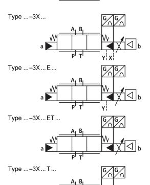
Symbol, detailed (pilot oil supply and pilot oil drain external)
