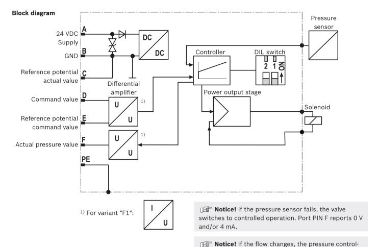
ler is automatically adjusted to these operating conditions. In the first cycles, this may lead to changes in the transition behavior.
