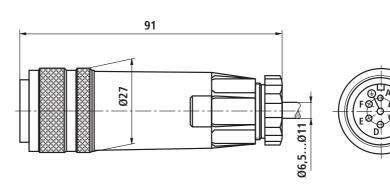
Cable socket (metal version) to DIN EN 175201-804 Separate order, material no. R900223890
