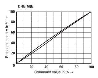
With valve DRE(M), the manufacturing tolerance at the external amplifier (type and data sheet see page 2) can be changed using the command value attenuator potentiometer "Gw". With the digital amplifier, the setting is made using the "Limit" parameter.
