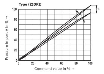
With type (Z)DRE, the manufacturing tolerance at the external amplifier (type and data sheet see page 7) can be adjusted using the command value attenuator potentiometer "Gw". Digital amplifiers are adjusted using the parameter "Limit".
