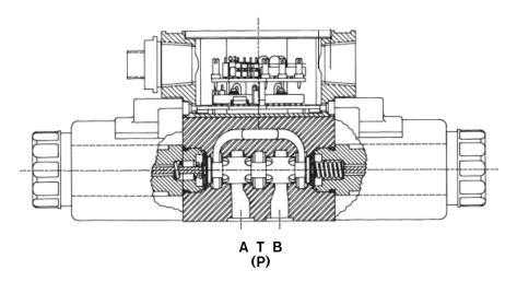
Proportional directional control valves Model 4 WRA B 6 and 4 WRAE B 6 are direct operated spool valves. They control the direction and quantity of flow to an actuator, for smooth acceleration to a desired velocity. The valve is normally operated by integrated electronics or a suitable amplifier. The 4 WRA B can be operated as a switching valve if proportional control is not required.
