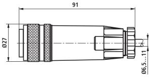
Plug-in connector to DIN EN 175201-804 Separate order: Material No. R900223890 (metal version)
