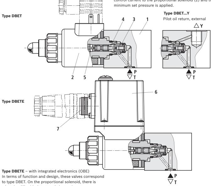
a housing (6) with the control electronics.
