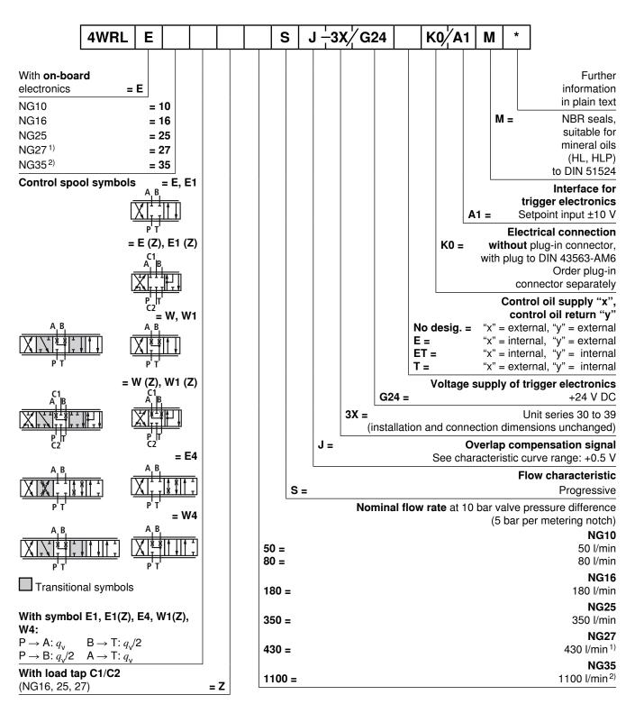
$<sup>^{1)}</sup>$  NG27 is a high-flow version of NG25, ports P, A, B and T have Ø 32 mm in the main stage. Contrary to standard ISO 4401-08-08-0-05, ports P, A, B and T may be drilled to max. Ø 30 mm in the control block. These valves therefore offer higher flow rates  $Q_{\rm A}$ :  $Q_{\rm B}$
