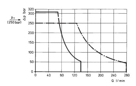
$\begin{array}{l} \textbf{Doubled flow rate} \\ p_{\text{max}} = 250 \text{ bar} \end{array}$
