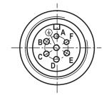
Mating connector according to DIN EN 175201-804 separate order under the Material no. **R900223890** (metal version)
