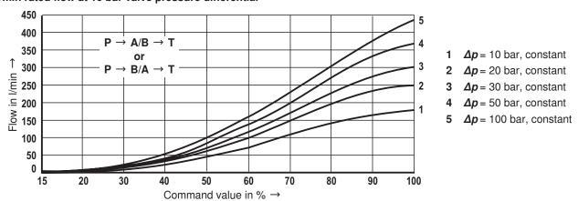
$\Delta p$  = valve pressure differential according to DIN 24311 (inlet pressure  $p_p$  minus load pressure  $p_1$  minus return flow pressure  $p_T$ )
