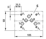
Valve mounting screws (separate order)
