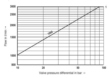
Recommended flow limitation (flow velocity 30 m/s) in the valve connection bores
