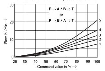
15 I/min nominal flow at 10 bar valve pressure differential
