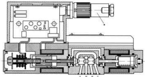
Control solenoid with position transducer
