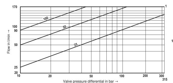
1 = Recommended flow limitation (flow velocity 30 m/s) in the valve connection bores
