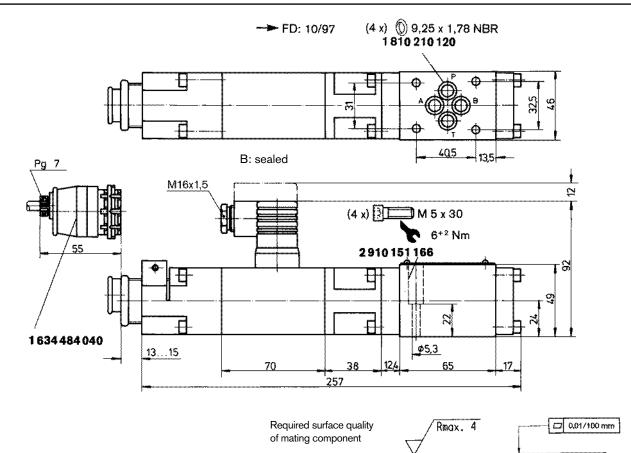
Mounting hole configuration: NG6 (ISO 4401-03-02-0-94) For subplates, see catalog sheet RE 45053
