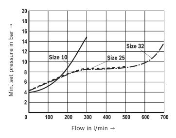
The characteristic curves apply to output pressure in T or Y = 0 bar in the total flow range.
