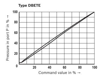
1) With valve type DBET, the manufacturing tolerance at the **external amplifier** (type and data sheet, see page 14) can be changed using the command value attenuator potentiometer "**Gw**". The digital amplifier is set using the parameter "Limit".
