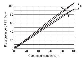
1) For valve ZDRE the tolerance can be modified on the external amplifier (for type and data sheet, see page 2) using command value attenuator potentiometer "Gw". The digital amplifier can be adjusted by means of parameter "Limit".
