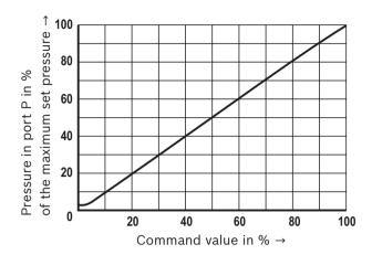
Minimum set pressure in port P with command value 0 V and/or 4 mA depending on the flow (return flow pressure = 0 bar)
